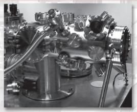
Preparation chamber with various flanges for evaporation cells, sputter sources, LEED etc.
